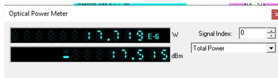
GAMBAR 5. PENGUKURAN DAYA DI PERANGKAT ONT TERDEKAT PADA FEEDER OLT 1
