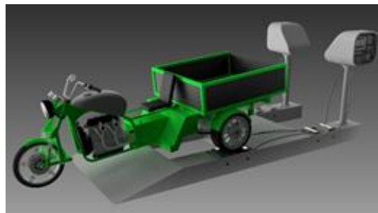
GAMBAR 1. SKEMA UJI ENGINE DI CHASSIS DYNAMOMETER
