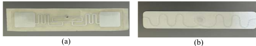
GAMBAR 3. Tag RFID (a) Chip Alien H3 and (b) Chip NXP Ucode 7
