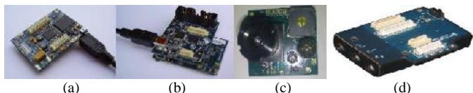
Gambar. 2 (a) radio processor board (IPR2400) [11] (b) interface board [11] (c) sensor board (IMB400) [8] (d) power supply board (IBB2400) [12].
