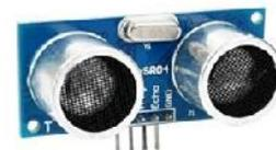
Gambar 4. Sensor Jarak HC-SR 04
