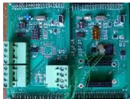
Gambar 8. Extended Module Board Analog I/O
