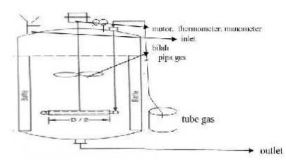
Figure 2 Biogas reactor or bioreactor
