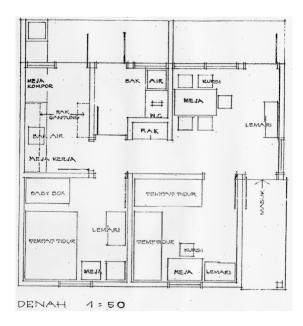
Gambar 4: Gambar Denah R.S. T.36
