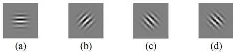
Gambar 9: Tapis Gabor 2-D bagian imaginary berukuran 33 \times 33 (a) 90^\circ (b) 45^\circ (c) 0^\circ (d) -45^\circ
