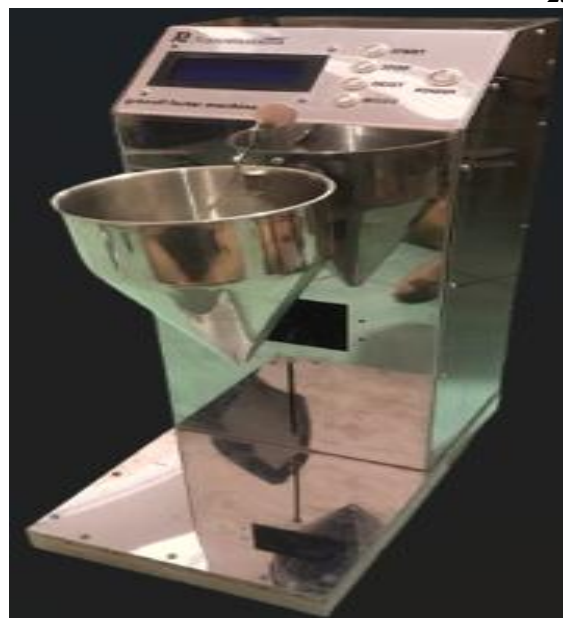
Figure 4. Front view of granule testing equipment granule holder before testing the flow time and a holder for the sensor, solenoid and infrared proximity sensor.
