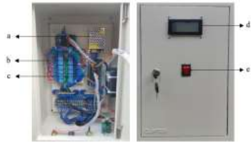
Figure 7: Pool Water Quality Control Circuit in Panel.
