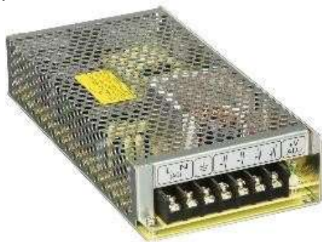
Gambar 3: Power Supply Switching
