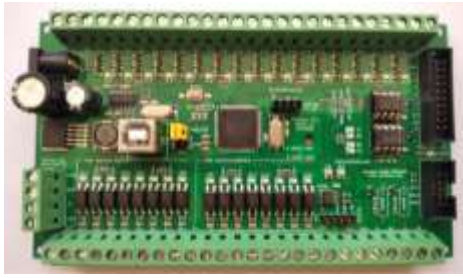
Gambar 1: Outseal PLC Mega V.3 Standar PP
