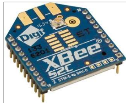
Figure 2: Physical Form the XBee S2C
