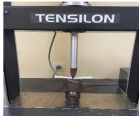
Gambar 2. Proses pengujian bending
