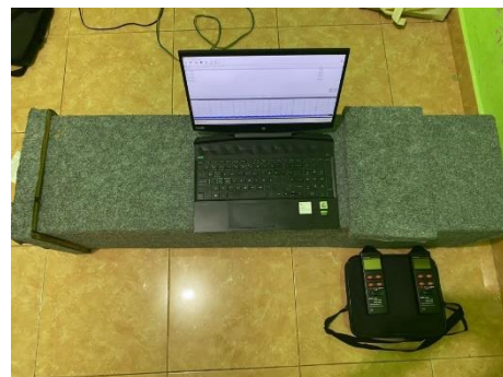
Gambar 2. Proses pengujian transmission loss
