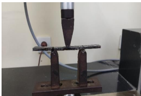
Gambar 2. Proses pengujian bending
