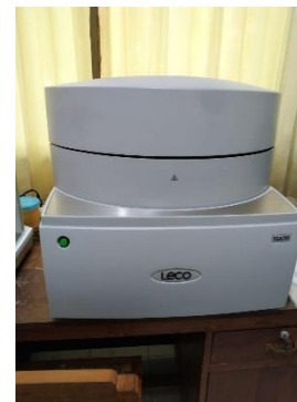
Gambar 1. Alat uji Proximate
