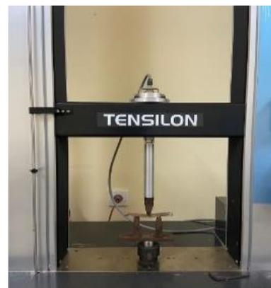
Gambar 7. Proses uji bending
