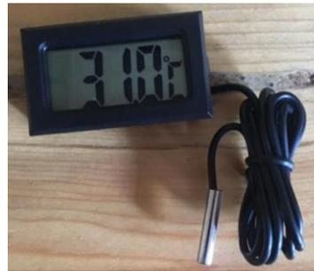
Gambar 3. Termometer digital
