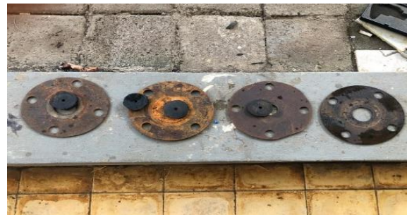
Gambar 3. Variasi diameter lubang katup limbah 26 mm, 31 mm, 36 mm, 41 mm, dan 46 mm
