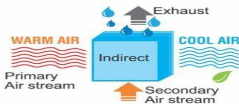
Gambar 1. Prinsip Kerja Sistim Indirect Evaporative Cooling
