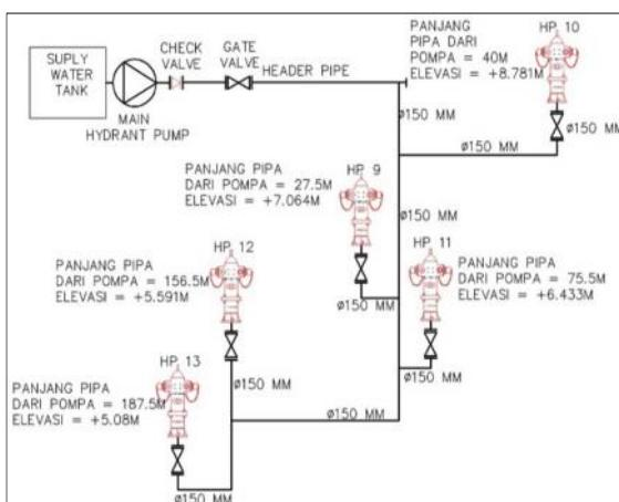
Gambar 3. Skema instalasi fire hydrant zona 3
