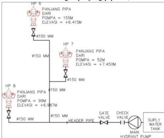
Gambar 2. Skema instalasi fire hydrant zona 2
