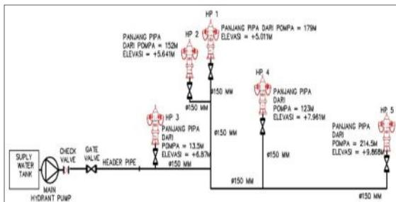
Gambar 1. Skema instalasi fire hydrant zona 1
