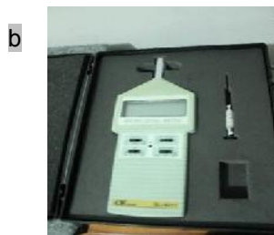
Gambar 1 a. alat Uji Transmission loss , b. Sound Level Meter (SL-4011).
