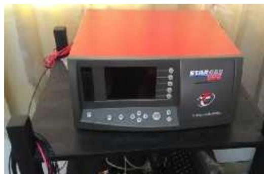
Gambar 2 Alat ukur emisi gas buang Stargas model 898
