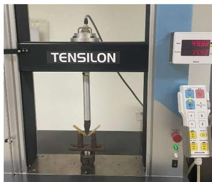
Gambar 4. Proses Uji Bending
