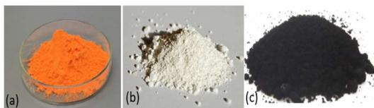
Gambar 2. (a) H<sub>2</sub>PtCl<sub>6</sub>, (b) TiO<sub>2</sub>, dan (c) Vulcan XC-72
