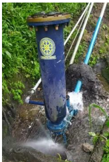
Gambar 1. Prototype pompa hidram dilapangan
