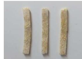
**Gambar 6. Benda Uji Impak**
