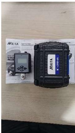
Gambar 4. Torque Gauge
