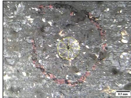
Gambar 7. Lebar Diameter Indentasi 0,595 mm
