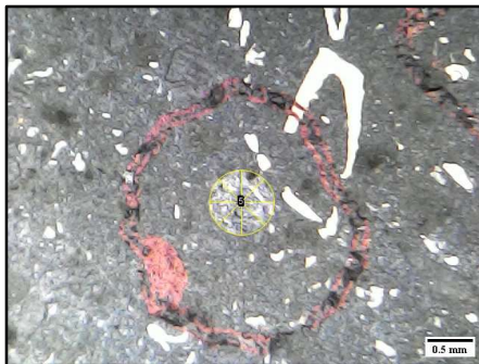
Gambar 5. Lebar Diameter Indentasi 0,514 mm
