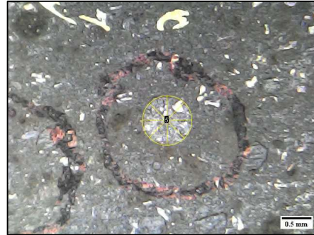
Gambar 6. Lebar Diameter Indentasi 0,547 mm
