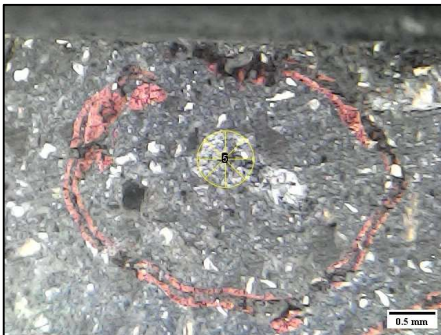
Gambar 3. Lebar Diameter Indentasi 0,419 mm
