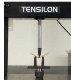
Gambar 4 Proses Uji Bending
