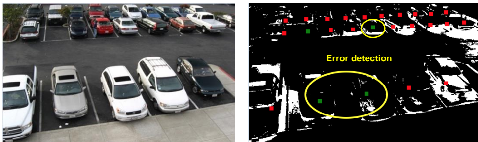
Figure 8. Illustration of an Occupied Parking Lot Detection Error
