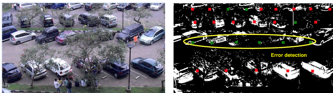
Figure 11. Example of Errors Detection at MOG Parking Area
