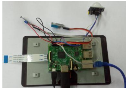
Figure 3. Raspberry pi 3 model B which is connected with three sensors
