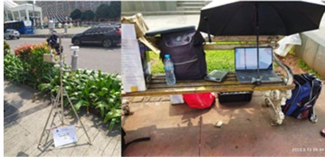
Gambar 2. Serangkaian Alat Mini Weather Station
