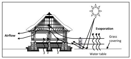
Figure 5: Creating comfortable Internal Environment
