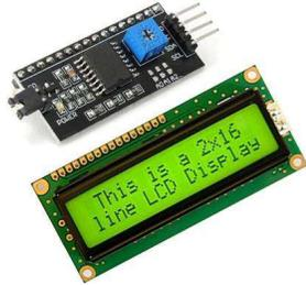
Gambar 4: LCD 16x2 + I2C
