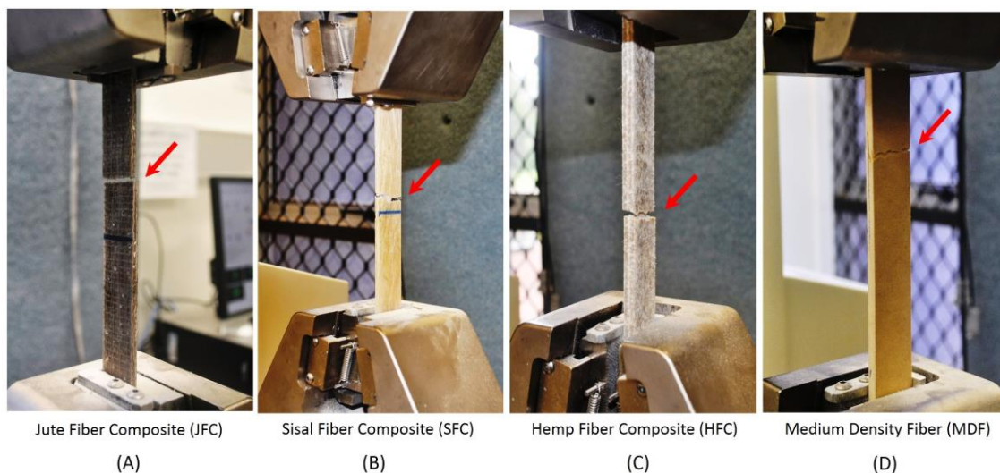
Figure 3. Failure mode of lignocellulosic composites under tensile load; (A) Jute fiber composite, (B) Sisal fiber composite, (C) Hemp fiber composite, and (D) Medium density fiber
