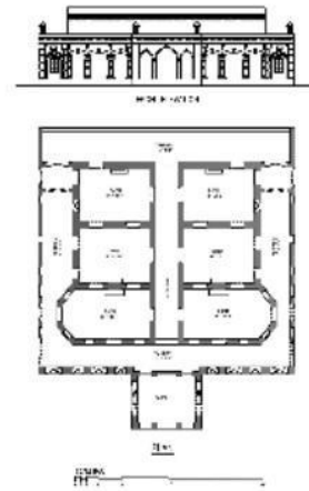
Picture 6: Layout of a bungalow with central corridors and symmetrical rooms on both sides
