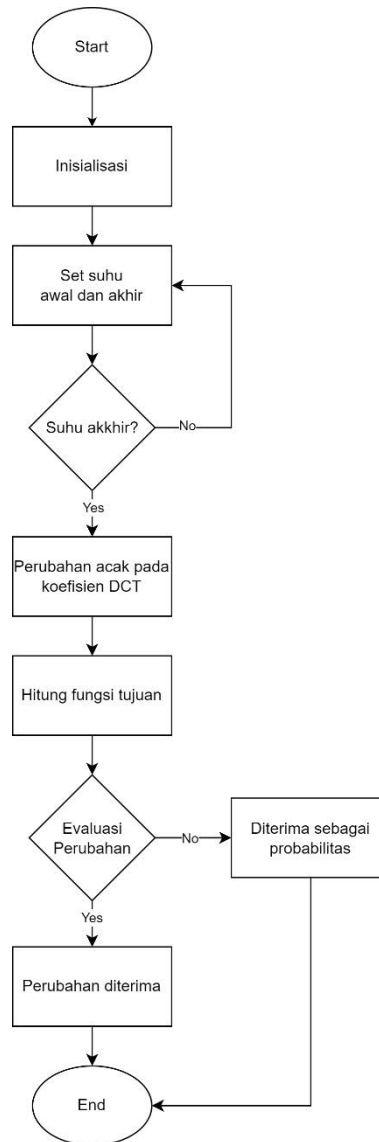
Gambar 3. Flowchart Algoritma Simulated Annealing
