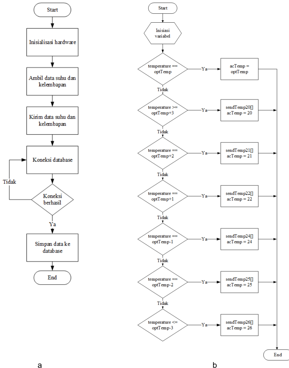
Gambar 2. Flowchart Penyimpanan Data (a), Flowchart Pengiriman Sinyal Infrared Transmitter (b)
