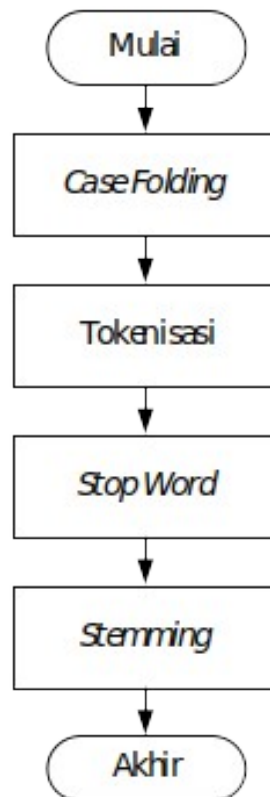
Gambar 2. Diagram Alur Preprocessing Pesan
