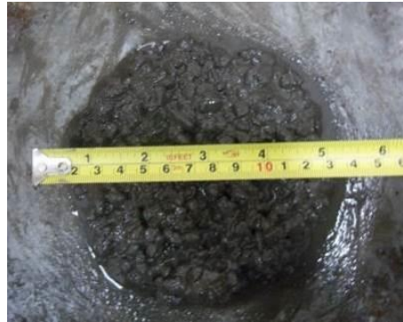
Gambar 18. Flow test Beton Geopolimer
