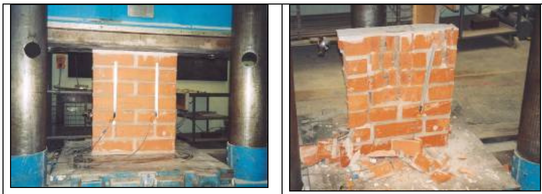
Figure 1. Typical rectangular wallettes of clay brick prisms before and after testing
