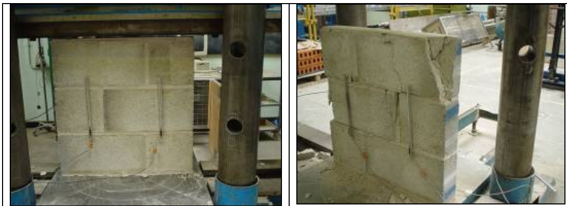
Figure 3. Typical rectangular wallettes of concrete block prisms before and after testing
