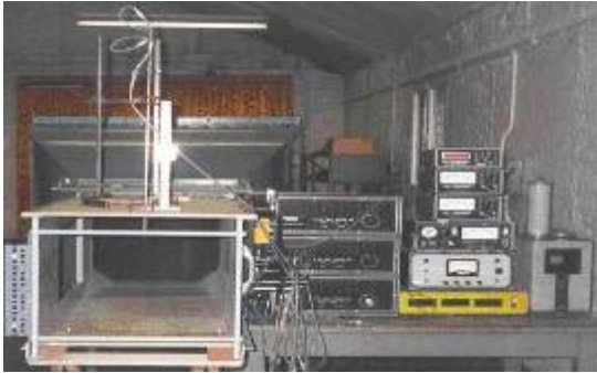
Figure 10c. Photo Small Wind Tunnel (Department Marine and Technology)
