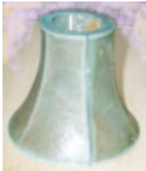
Figure 6a. 1:1000 Scale Model of Single Cooling Tower
