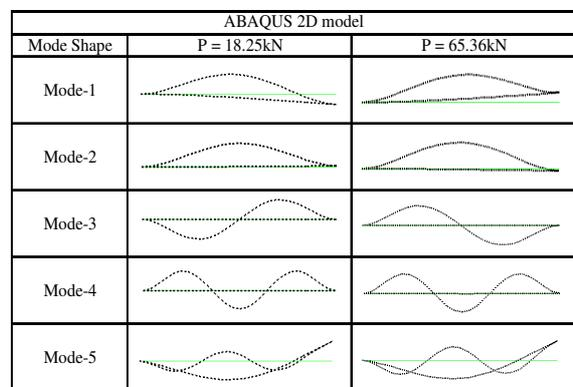
**Figure 7. Mode shapes of a post-tensioned masonry column, ABAQUS 2D Model**
