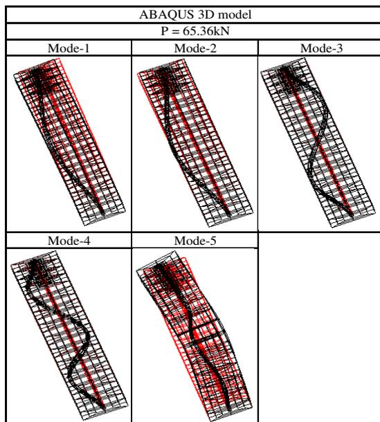
Figure 8. Mode shapes of a post-tensioned masonry column, ABAQUS 3D Model
