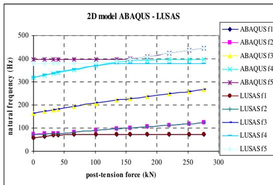
**Figure 10. Comparison between natural frequencies 2D Models ABAQUS and LUSAS**
