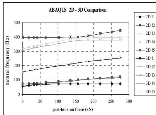
Figure 9. Comparison between natural frequencies ABAQUS 2D and 3D Models
