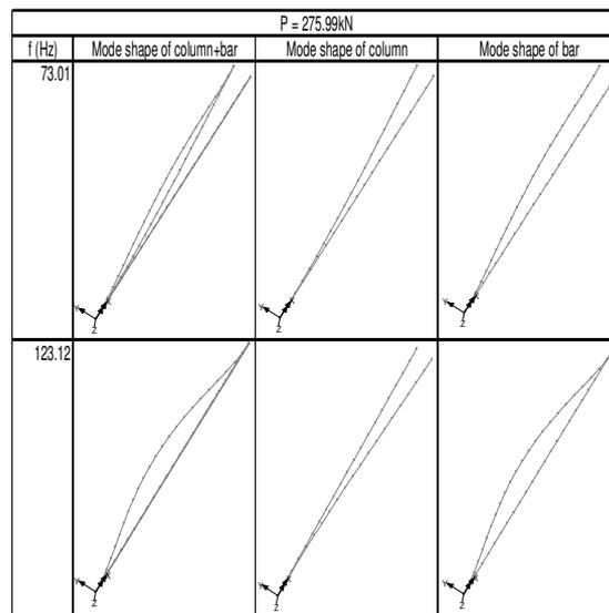
**Figure 4. Mode shapes of a post-tensioned masonry column - LUSAS 2D Model**
