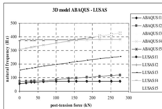
**Figure 11. Comparison between natural frequencies 3D Models ABAQUS and LUSAS**
