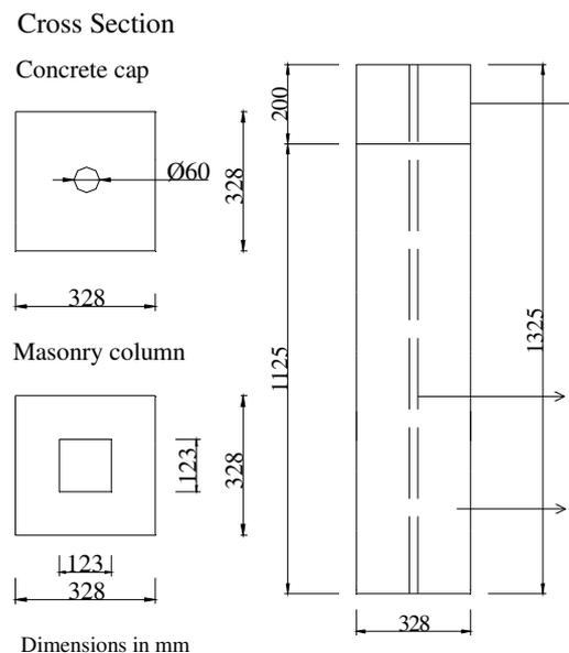
**Figure 1. Plan and elevation of post-tensioned masonry column**
