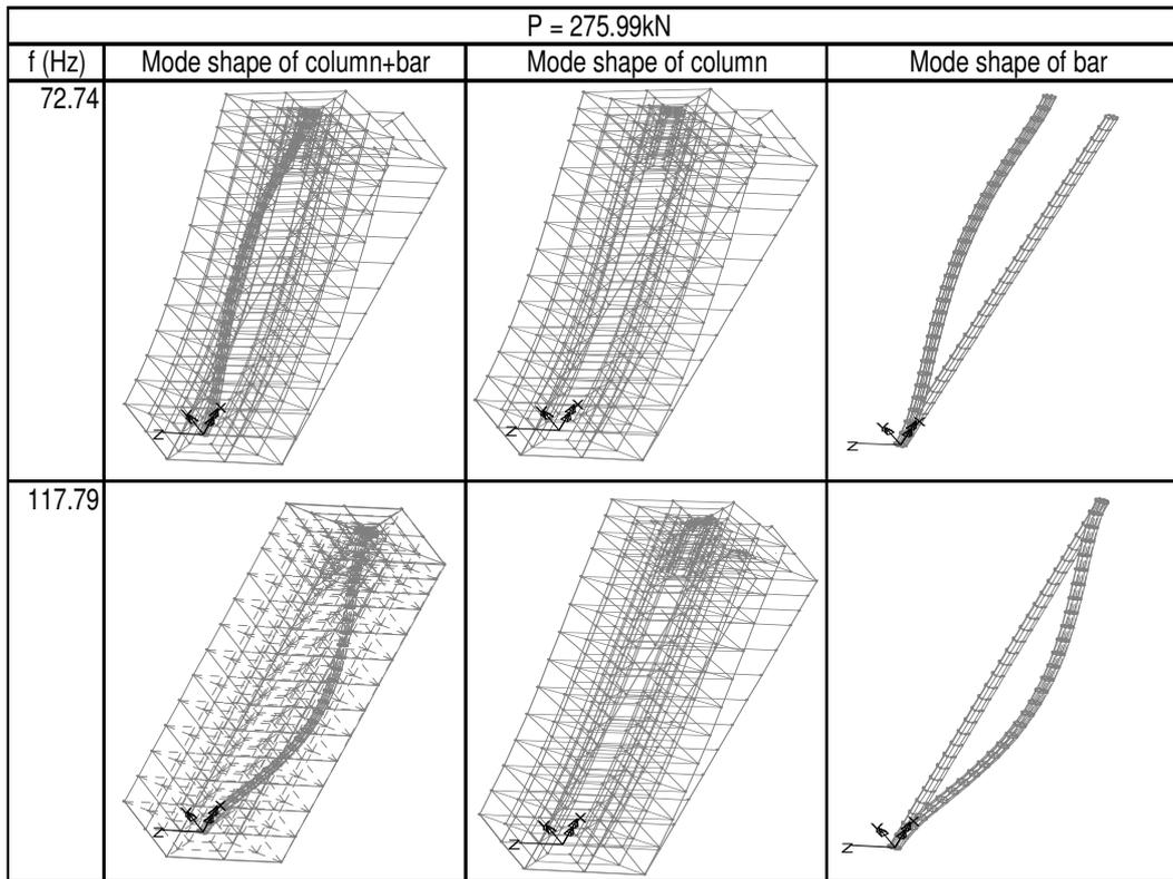
Figure 5. Mode shapes of a post-tensioned masonry column- LUSAS 3D Model
