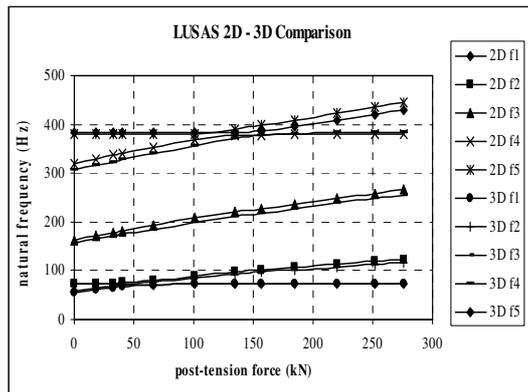
**Figure 6. Comparison between natural frequencies LUSAS 2D and 3D Models**
