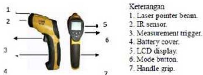
Gambar 7. Infrared Thermograf
