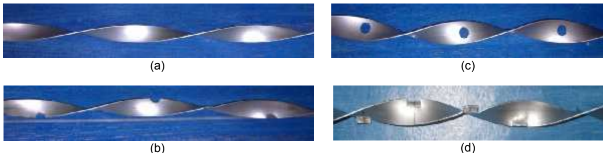
Gambar 3. Variasi twisted tape insert a.) Classic twisted tape insert ; b.) Notched twisted tape insert ; c.) Perforated twisted tape insert ; d.) Jagged twisted tape insert
