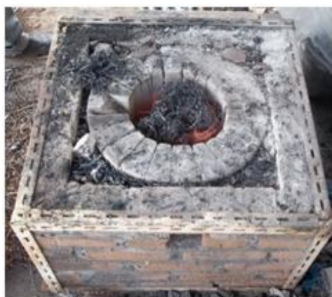
Gambar 4. Proses pelunakan limbah gram besi
