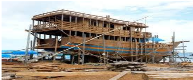
Gambar 1a Kapal Layar Phinisi proses finishing.
