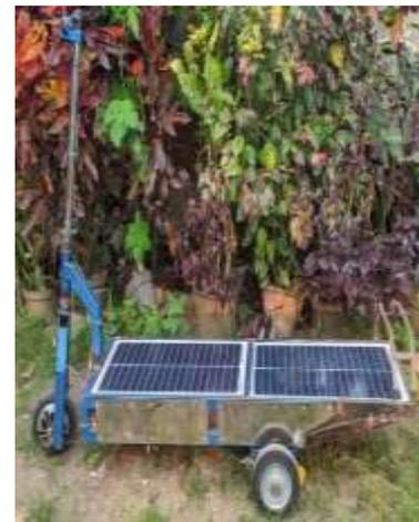
Gambar 5. Rangka *e-scooter* angkut
