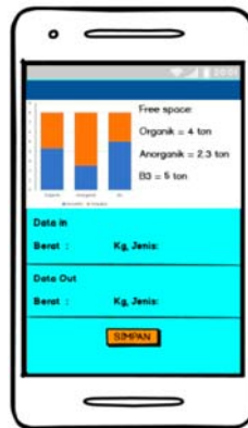
Fig. 11. TPA Officer Interface On this page the TPA Officer can only add incoming or outgoing data. The data will be stored in a database which can later be used as a source of free space information at a TPA so that if a TPS Officer wants to send waste to a TPA it can be sent to a TPA that still has sufficient free space.
