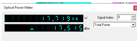
Fig. 5 Power Measurement in the nearest ONT device on the OLT 1 feeder
